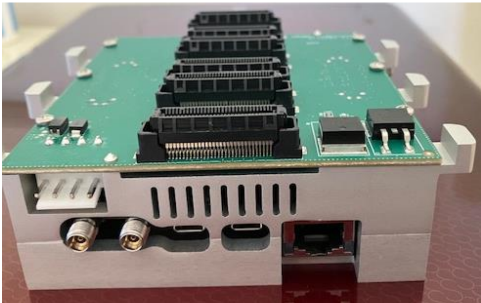
Figure 7: OT6000 backplane front view: Diff clock inputs 2.92mm; Ethernet; 12V Power and USB for debugging
